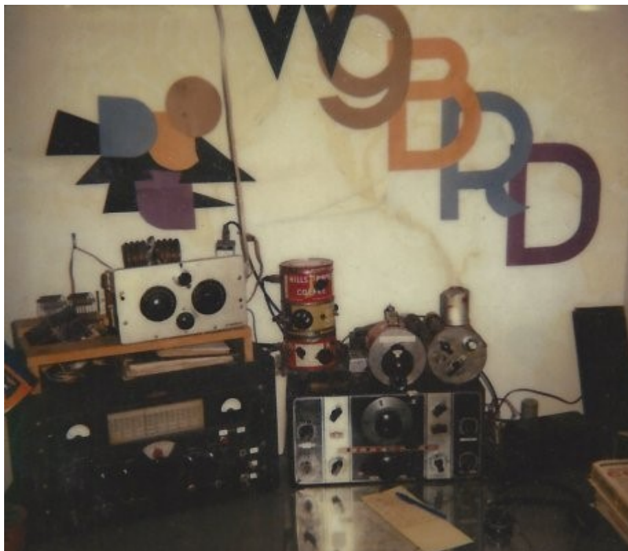
Figure 2 —"Studio 2"—my father's upstairs station for 40, 20 and 15 meters—of amateur radio station W9BRD III of the early 1980s CE. The Collins 32V-3 transmitter (left) was originally owned by his brother-in-law, Phil Simmons, W9VES. The receiver is a modified National NC-100X teamed with a two-Prince-Albert-cans regenerative converter originally built for use with the Hallicrafters SX-24 receiver used by W9VES until Phil's death in 1969; later in 1969 the NC-100X and converter would serve as my receiver at Novice amateur radio station WN9CJS. Note not only the cool stylized W9BRD sign, but dad's use of the resulting paper cutouts to form the birdlike collage to its left. (The water stain is on the photo, not the station wall!)
